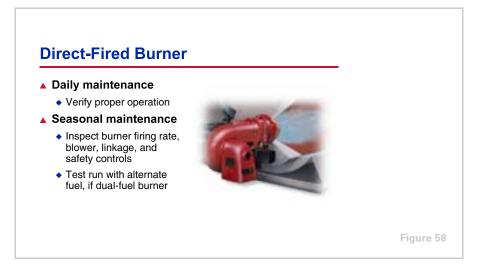
The burner is the heart of a direct-fired absorption chiller. Correct operation is, therefore, necessary for optimum chiller performance. Daily checks should be made in accordance with the manufacturer's recommendations. Each cooling season, the burner's firing rate, blower, linkage, and safety controls should be checked to ensure proper operation. If a dual-fuel burner is being used, it should be periodically test run with the alternate fuel to ensure reliable operation.
